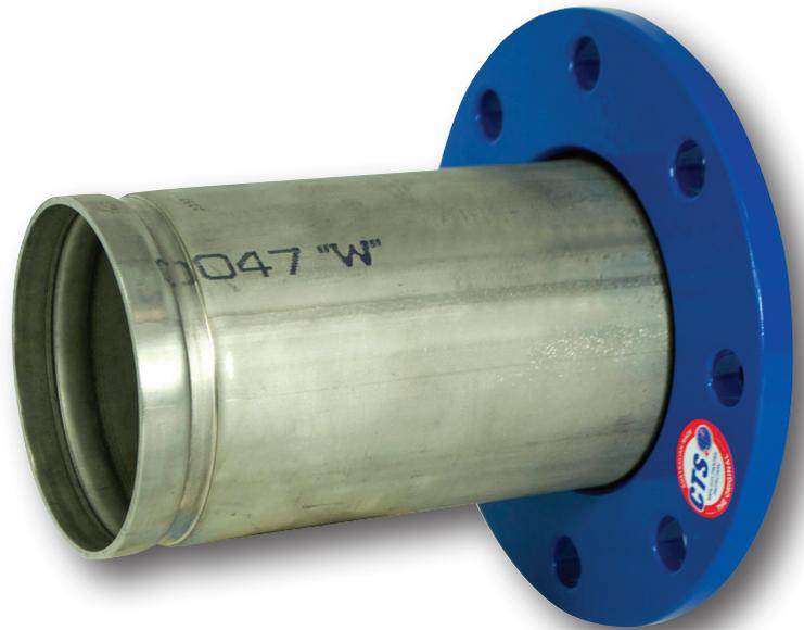
CTS HVAC-R now offer another innovative pipe line solution. The CTS Roll Grooved to Flanged Pipe Spool enables easy connection from a Flange to a component, with a roll groove end incorporated in the one integral unit. Designed for HVAC and civil water piping systems, the CTS RG Spool negates costly onsite fabrication.
